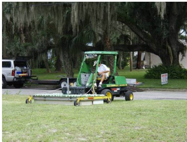
Figure 5. Radar tomography survey. Photograph by author.
