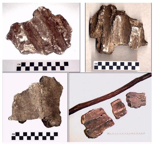
Figure 17. Tabby Daub from Cabin #1. Samples Showing Smoothly Finished Surface and Vine Impressions. Example of Local Grape Vine, Lower Right.
